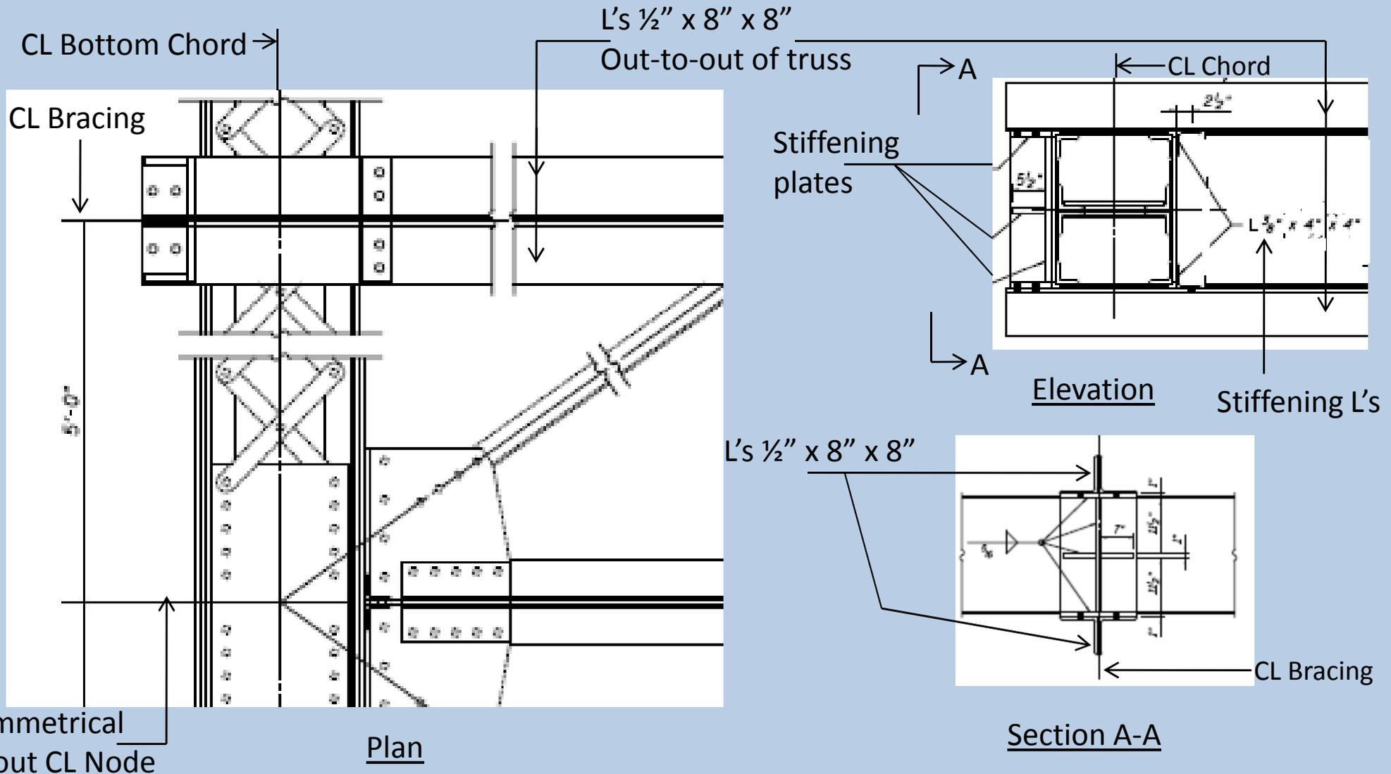
Note: Full system for this node includes two sets of lateral bracing – one on each side of the node. Each set runs from out-to-out of the truss. Also strengthened a diagonal brace. The dead load force in the bottom chord is 975 k.
